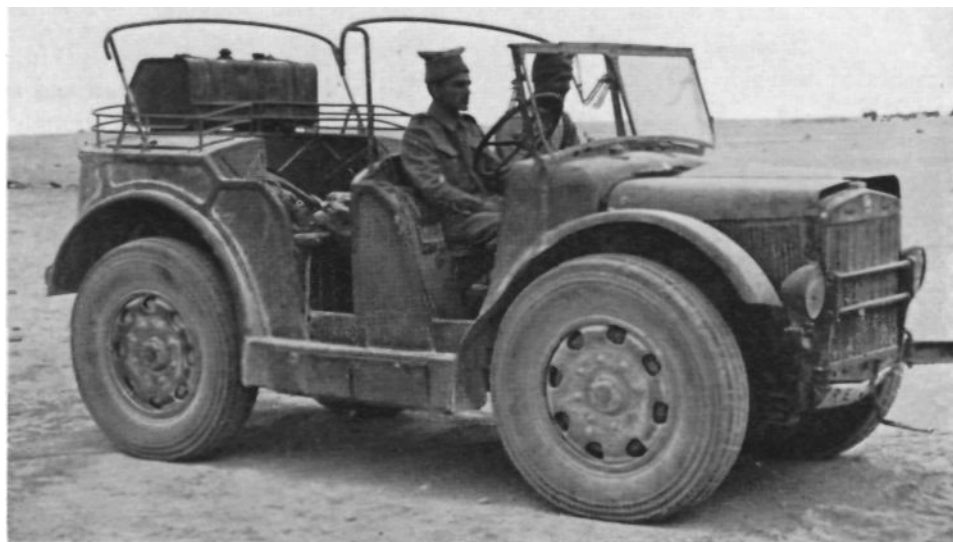
For desert use the Italians have developed a stubby staff car with a high degree of flotation. The boxed-in running boards form lockers for tools or equipment. Crank and high position of gas tank indicate that self-starters and fuel pumps are unessential luxuries. (British Press Service photo)
