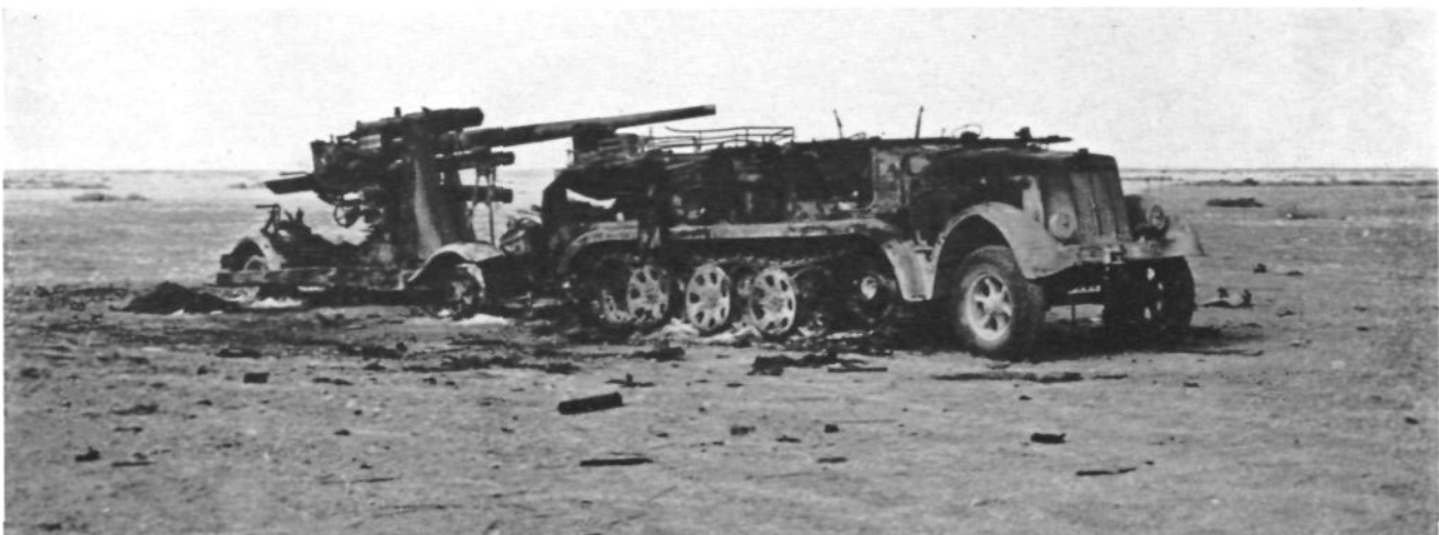
"It can produce a big punch." This German 88-mm. AA and AT gun was on the receiving end in Libya. Like nearly all AA guns with the field army, it is fitted with a shield for protection during AT action. The prime mover is the standard medium half-track used for many different purposes.
