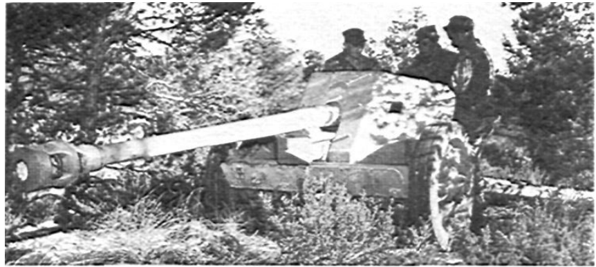
PAK 40, 75-mm in caliber, looks like an overgrown 50-mm PAK 38, with its tubular split trail, double shield, extremely low silhouette, etc. Its enormous powder chamber extends practically to the shield, to accommodate the large propellant required to give a muzzle velocity of around 3,000 f/s. Much manufacturing time and cost are saved by leaving unimportant exterior surfaces rough, rather than machining them.
