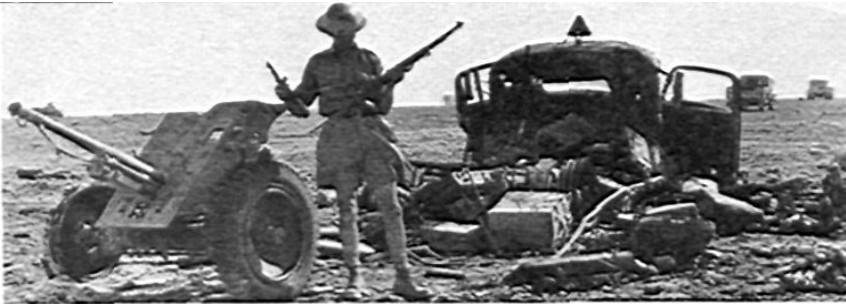
Germans call their AT guns PAK, meaning Panzer Abwehr Kanone. This 37-mm piece, which was towed by the burned-out truck, is of the type developed around 1934, proved in the Spanish Civil War, and sold throughout the world for foreign exchange. Our own 37 is patterned after this one.
