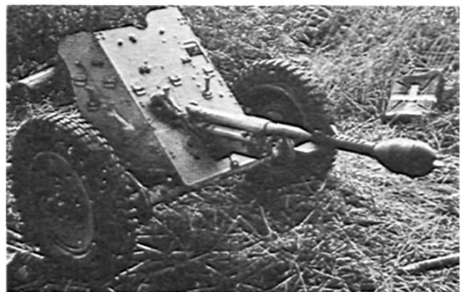
As tanks became more heavily armored the effective range of the little 37-mm shell (see bottom of photo) became shorter and shorter. Germany has pushed her 37-mm PAK right back to the forefront, however, by adopting a bulbous hollow-charge Stielgranate which is projected by a blank charge. Terminal velocity is of practically no importance, so effectiveness is limited only by (1) accuracy (the ability to hit the target with this somewhat unwieldy projectile) and (2) the explosive power of the particular grenade that is used.
