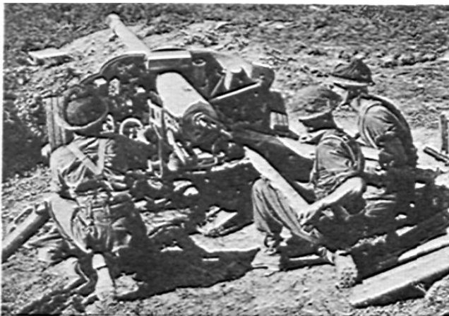
As is often mentioned, Germans are adept at adapting foreign materiel to their own use; here is some proof. A standard French 75-mm gun (fitted with a muzzle brake) has been mounted on a PAK 38 (5-cm AT) carriage. This combination is called the PAK 97-39. This one seems to use standard ammunition, but in many cases foreign guns have been rechambered for higher muzzle velocities.
