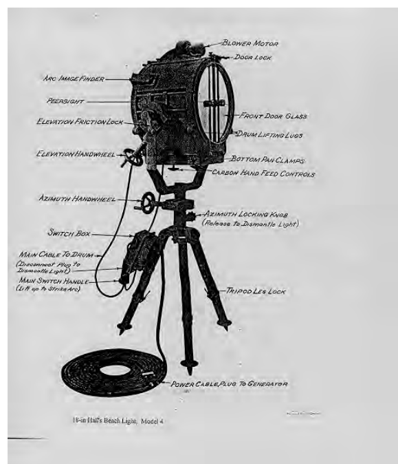
Figure 30: Typical searchlights used on John Point and Mushroom Rocks Courtesy Robert Mitchell.
